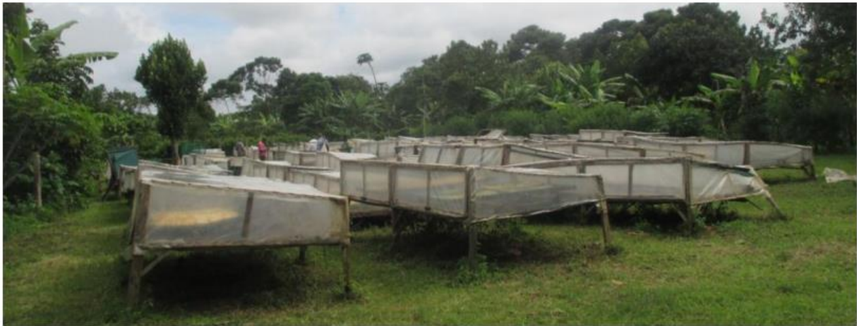
Static bed box type solar model dryer (Galyaki, C)
